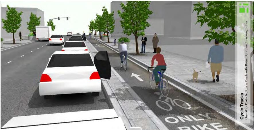
On-street bike lanes with a physical barrier separating the bike lane from motor vehicle traffic. The barrier can include flower planters, concrete curbs, plastic bollards, jersey barriers, and parked cars. Protected bike lanes can be either one-way or two-way.
