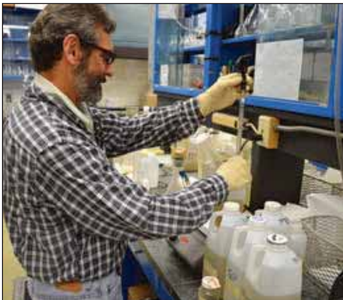
Scott Pierce, 3A operator/lab technician, runs a suspended solids test on the mixed liquor.
